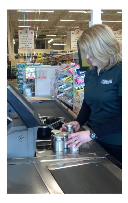
A Division Investigator testing a small capacity scale during an audit at a local grocery store.
