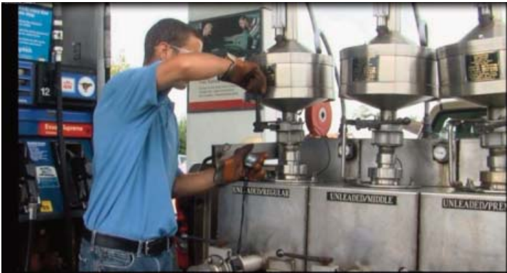
Figure 6 – Inspector Draining a Prover
