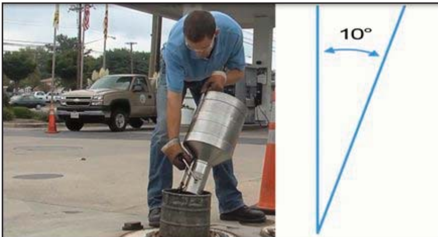
Figure 3 – Inspector Draining a Test Measure at a 10 Degree to 15 Degree Angle.
