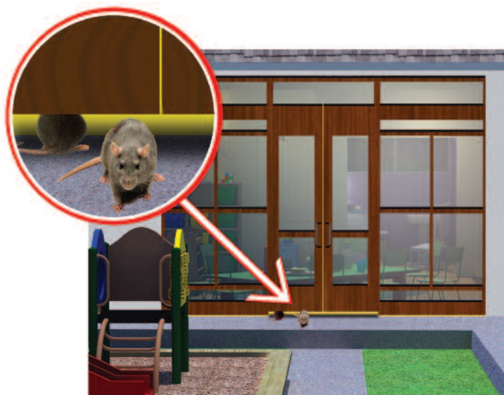
Install door sweeps.
