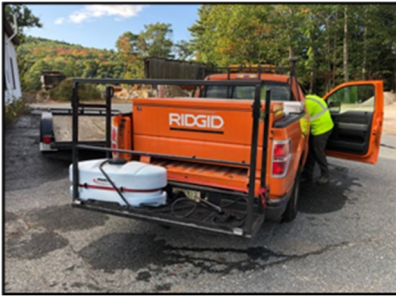
The DOT truck in the left-hand photo shows the 25-gallon tank spray and cone basket that Mr. Cygan uses while treating along highways, mostly for control of Japanese knotweed. Both photos on the right show treatment results.
